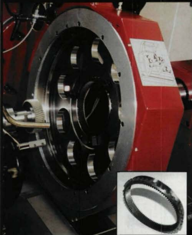
Honing of Automatic Transmission Ring Gear
