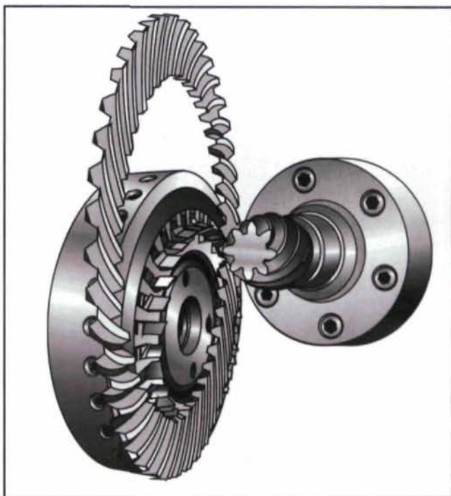
Figure 3—Circular cutting tool and virtual generating gear.
