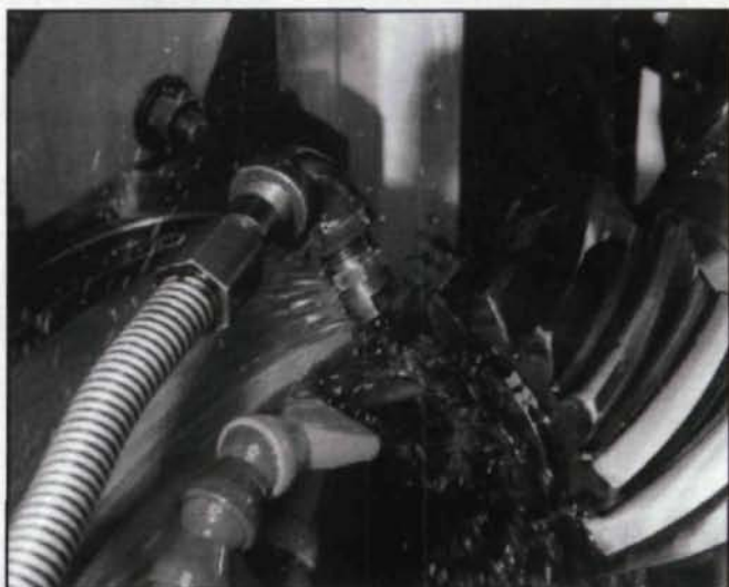
Figure 9—Grinding of a bevel pinion.
