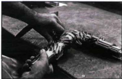
Fig. 1—Manual deburring is labor-intensive, inconsistent and expensive.
