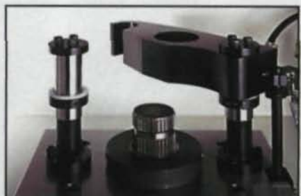
A short broach sticks out of the HS-100 deposit table and ring nozzle, below the machine tool's hold-down bar. The broach uses multiple up-and-down strokes to provide internal gears with the surface roughness of ground gears.
