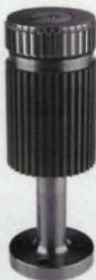
The short broach centers a gear with its upper set of teeth, then removes stock and flattens the gear's profile with the lower set of teeth.
