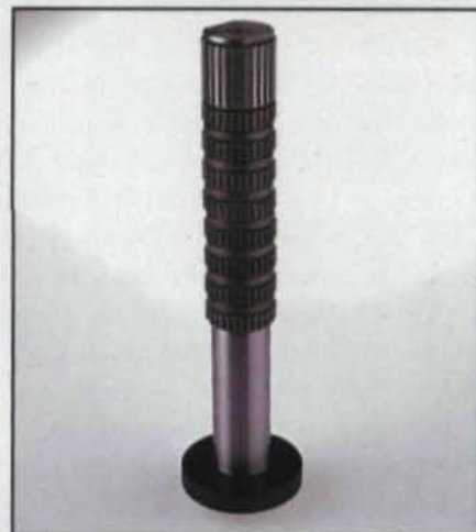
Fässler Corp.'s multiple-stroke short broaches, like this one, can finish-broach internal gears with small diameters and heat-treat distortion. A gear's major diameter can be as small as 20 mm.
