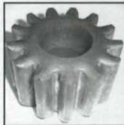
Figure 4—Through-extruded spur gear.
