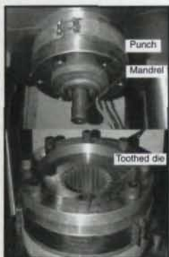
Figure 15—Photo of gear forging die.
