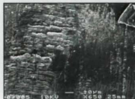
Figure 8—Typical surface topography of a PA66 gear running at 1,500 rpm and maximum contact stress of 39 MPa after 2.25 \times 10^6 cycles.
