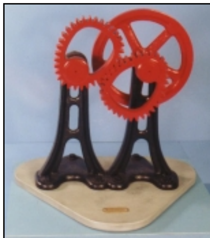
A chic red and black non-circular gear pair.
