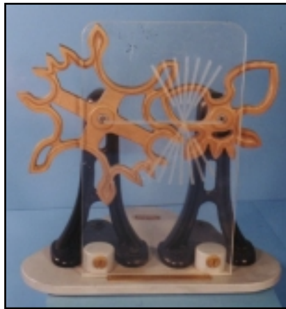
A variable pitch gear pair meshes compatibility.
