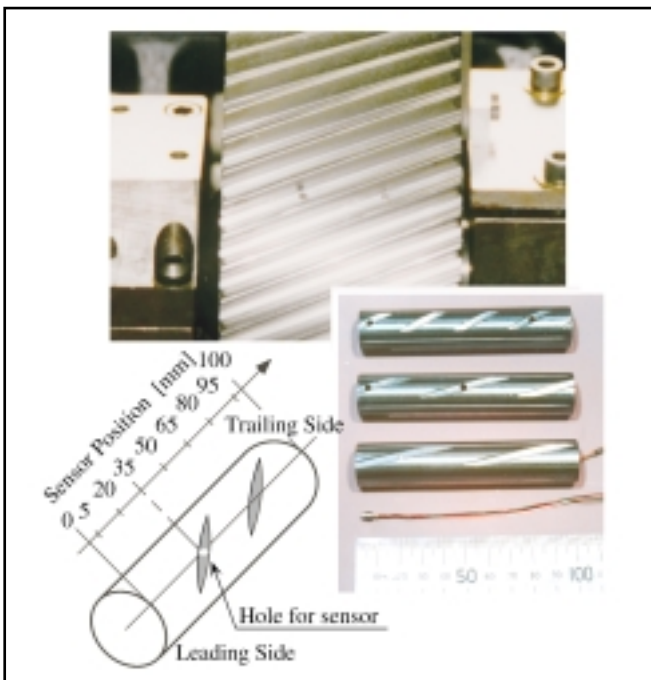
Figure 2—Appearance of rods and gear with rods at the bottom of teeth.
