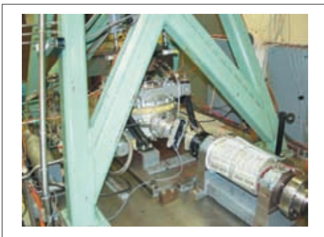
Figure 8—Static strain test setup.
