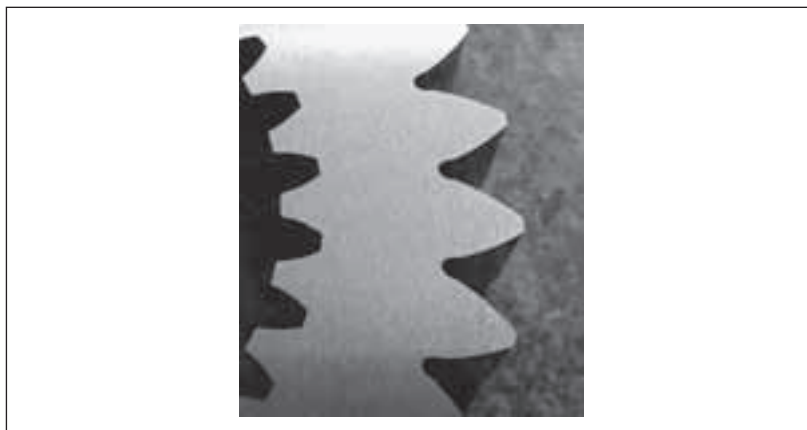
Figure 2—First-stage sun gear with asymmetric teeth.
