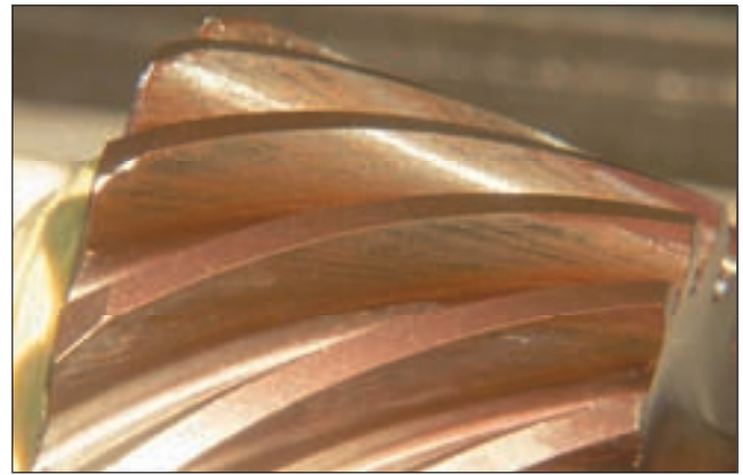
Figure 19—Spiral-bevel pinion tooth contact after tests. Formated design.
