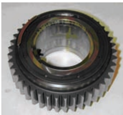
Figure 8—Second-stage sun gear.
