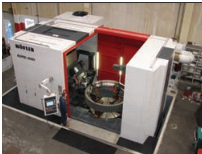
This Höfler Rapid 2600 gear grinder is one example of the specialized machinery necessary for wind turbine gear production. It can tooth grind gears up to 102” in diameter and weighing up to 20 tons. Placement of the 92,000-lb. machine requires a sunken foundation of 350 cubic yds. of reinforced concrete. The base of the foundation is supported by 12 auger cast pilings sunk to a depth of 50 ft. Photo courtesy of Seattle Gear Works.
