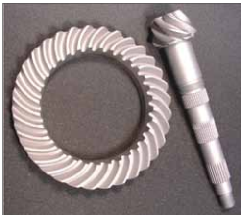
This ring and pinion set manufactured from the Ferrium C61 alloy has been employed in many off-road racing vehicles.
