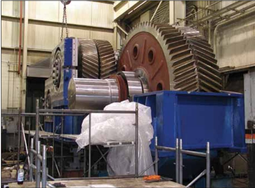
A complete rolling mill drive for an Eastern European client of Horsburgh & Scott had to be disassembled and packaged in individual parts for transportation (courtesy of Horsburgh & Scott).
