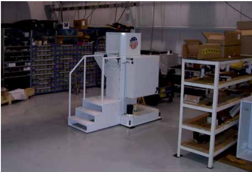
The Table Top Broaching Machine combines new concepts with traditional broaching methods in a smaller unit (courtesy of American Broach).
