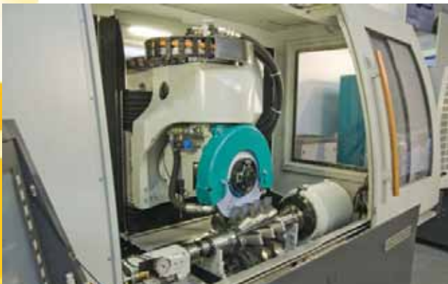
Schneeburger Large End Hob Grinder Up to 20" Diameter H obs with 20" Wheels. 52 Hp (100%) Power Plant.
