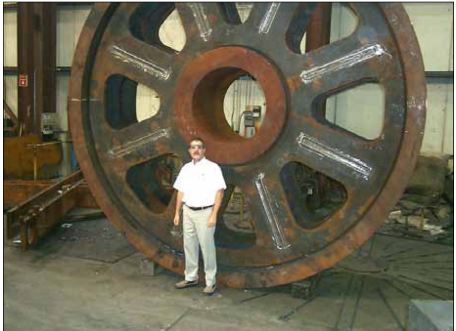
John Schnarr of HMC stands in front of a large fabricated gear for the steel industry (courtesy of HMC).
