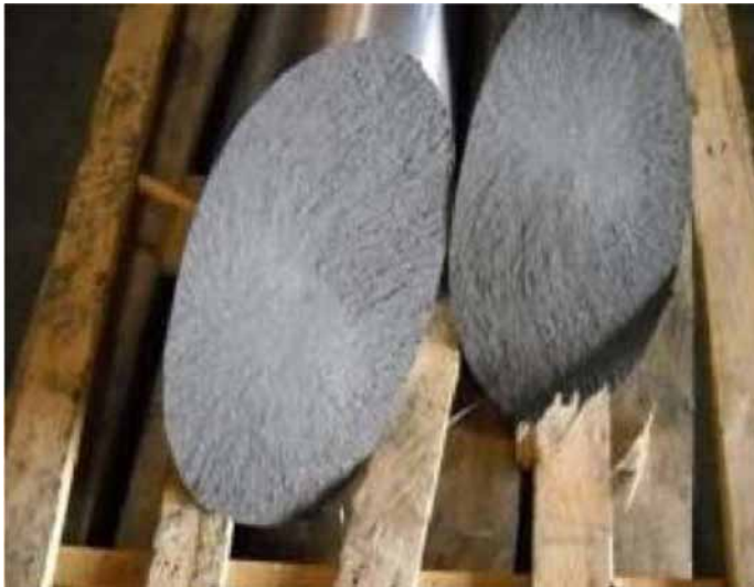
Figure 3—Sudden breakage due to hydrogen embrittlement.
