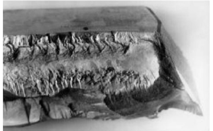
Figure 22—Magnification of the opposite edge of the broken surface.
