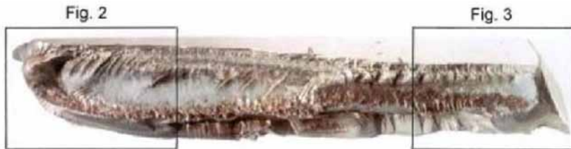
Figure 20—Example of fatigue fracture initiated from involute part of the profile.
