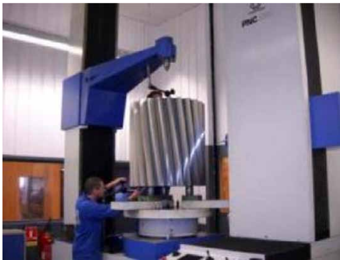
Figure 19—CNC gear measuring machine for heavy parts.
