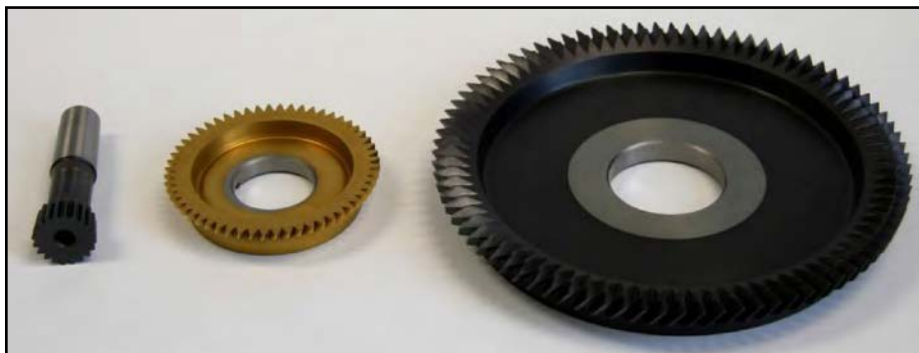
Figure 10 Solid HSS power skiving cutters coated with TiN and AlCrONite.
