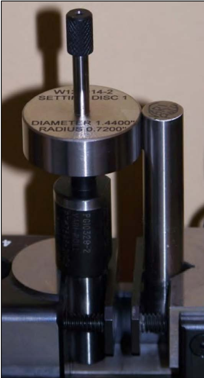
Figure 4 Calibration for tight mesh center distance (courtesy of Web Gear Services Ltd.).
