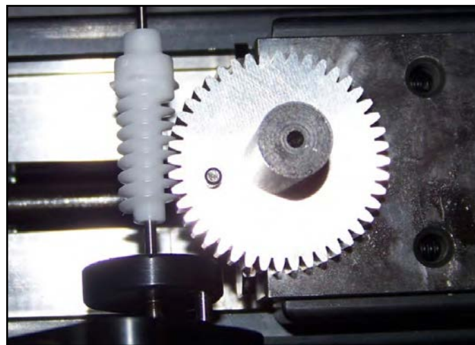
Figure 6 Plastic test worm in double-flank mesh with a master spur gear at an offset shaft angle (courtesy of Web Gear Services Ltd.).
