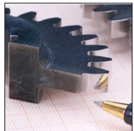
Figure 6 Near-mirror quality of a superfinished test gear.
