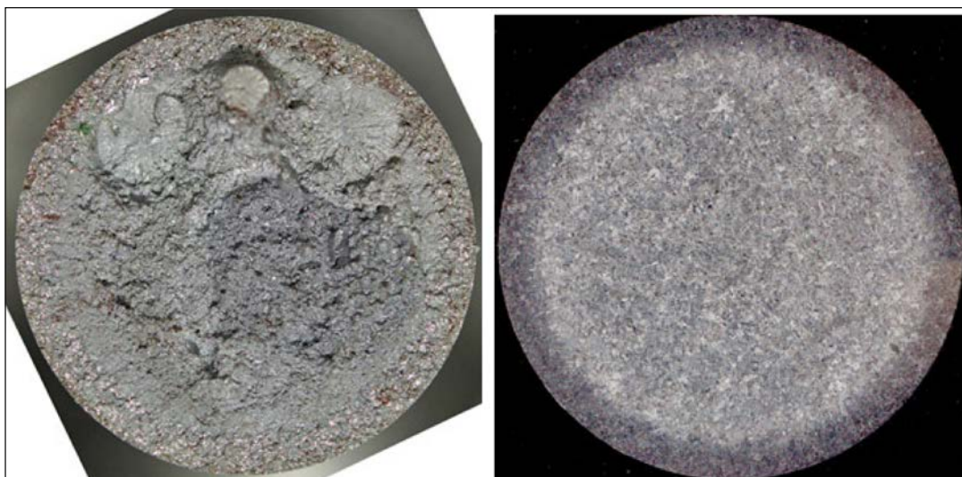
Figure 8 Segregation found in fatigue fracture surface and the polished and etched figure.
