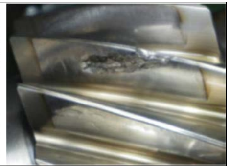
Figure 11 Cluster of impurity particles just under the tooth flank. Sudden spalling of tooth flank.
