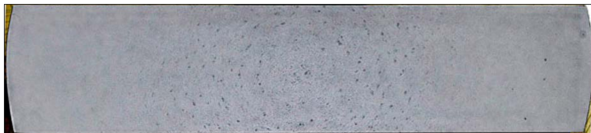
Figure 5 Macro-etched figure of a cross-section of CrMo steel bar of 800 mm diameter.
