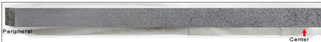
Figure 6 Macro-etched figure of 500 mm rectangular CrMo steel slab made by rolling.
