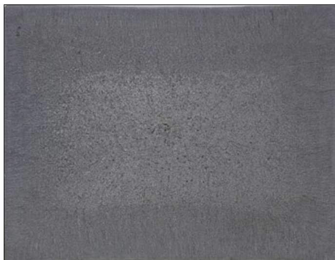
Figure 4 Cross-section of steel bloom just after congealed state in CC production.
