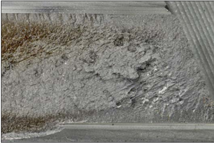
Figure 9 Cluster forming of impurity particles in gear steel.
