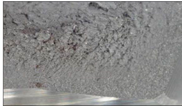
Figure 11 Cluster of impurity particles just under the tooth flank. Sudden spalling of tooth flank.
