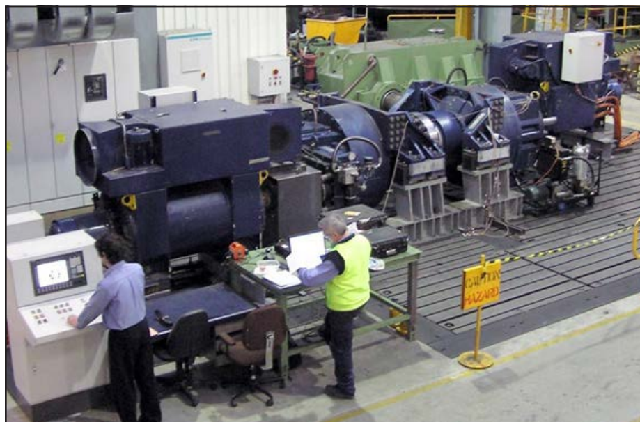
Figure 2 1MW-load GEARTest installation at Hoffman Engineering, Perth, Australia.
