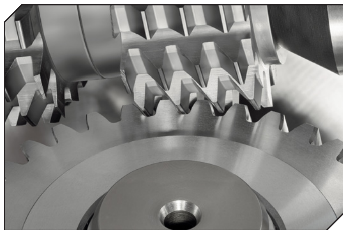
Chamfer hobbing for burr free flanks.
