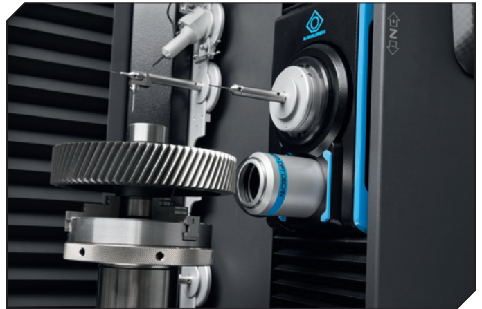
Figure 1 Pitch Measurement with HISPEED OPTOSCAN.
