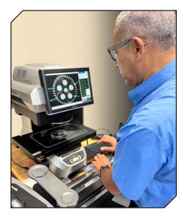
highly automated. For example, there is no time-consuming part positioning work or datum setup required. The simple "place-and-press" operation ensures consistent measurement of hundreds of dimensions on multiple parts with just the push of a button and regardless of operator skill.
