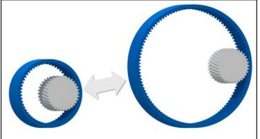
Figure 10 Variation in tooth root geometry and transmission ratio/teeth ratio.
