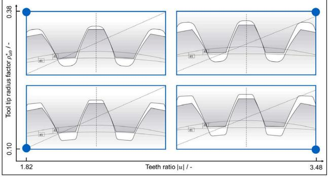
Figure 11 Gear variation with respect to teeth ratio and tool tip radius factor.
