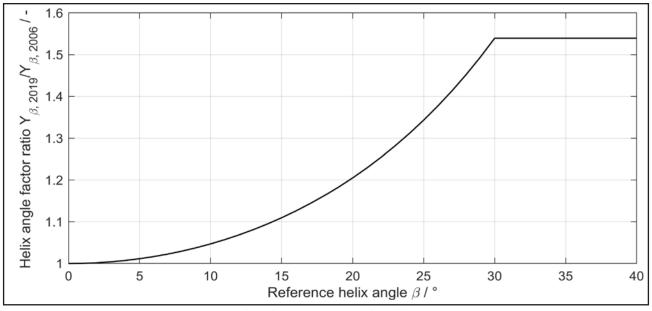
Figure 3 Helix angle factor ratio of ISO 6336-3:2019 (Ref. 1) and ISO 6336-3:2006 (Ref. 2).
