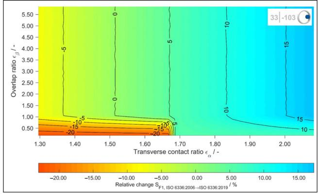
Figure 8 Relative change in the safety factor against tooth root breakage  $S_{FI}$  for the pinion, reference helix angle  $\beta = 25^{\circ}$ ,  $40 \times 40$  calculation points.
