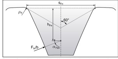
Figure 2 Geometrical variables at the critical section for internal gears according to ISO 6336-3:2019 (Ref. 1).
