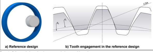
Figure 4 Reference design and tooth engagement in the external-internal gear stage.
