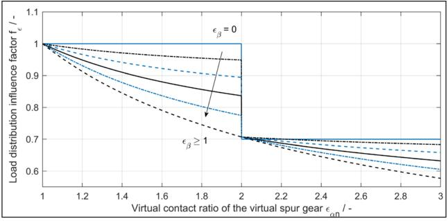
Figure 1 Load distribution influence factor according to ISO 6336-3:2019 (Ref. 1).
