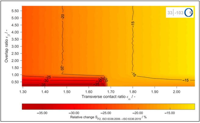
Figure 9 Relative change in the safety factor against tooth root breakage  $S_{F2}$  for the wheel, reference helix angle  $\beta = 25^{\circ}$ , 40 × 40 calculation points.
