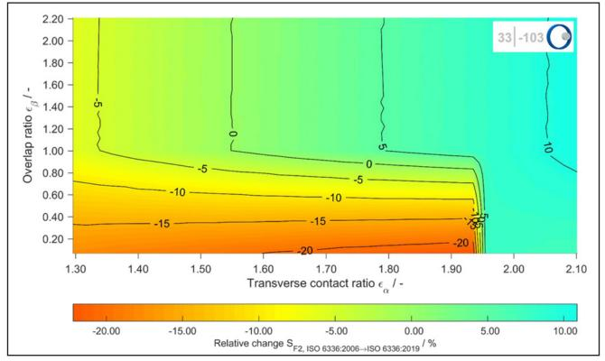
Figure 7 Relative change in the safety factor against tooth root breakage  $S_{F2}$  for the wheel, 40 × 40 calculation points.
