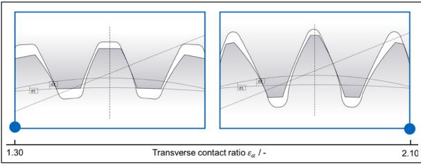
Figure 5 Gear variation with respect to transverse contact ratio.
