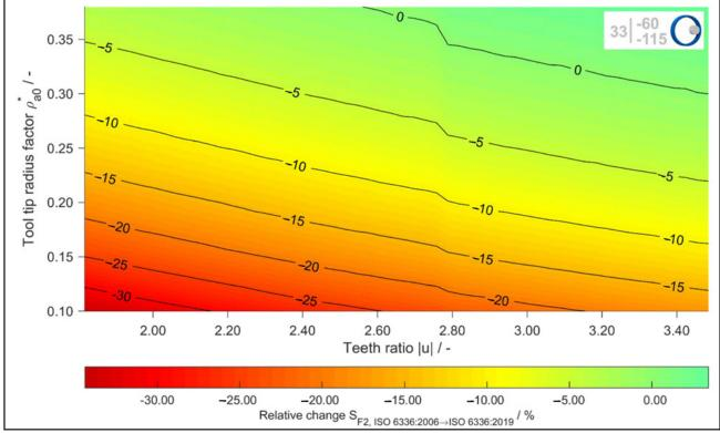
Figure 12 Relative change in the safety factor against tooth root breakage  $S_{r2}$  for the wheel, 56 × 40 calculation points.
