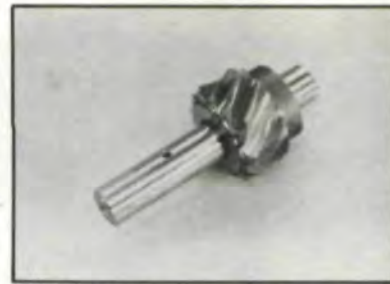
Fig. 15—Modified gear after 15 hours run
