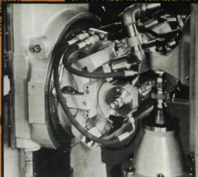
Fig. 1—Hobbing an external helical gear on a vertical gear hobber. Cutting action is produced by feeding the angular, gashed, worm-shaped hob through the gear blank in proper timed relationship. Courtesy Liebherr Machine Tool Div.
