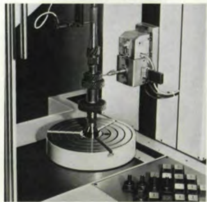
CNC controlled, 6 axis gear inspection machine
