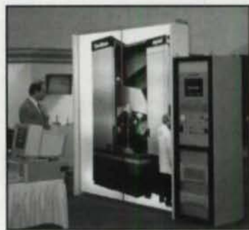
The OPAL 420 control system speeds grinding and changeover of Spur and Helical gears.
