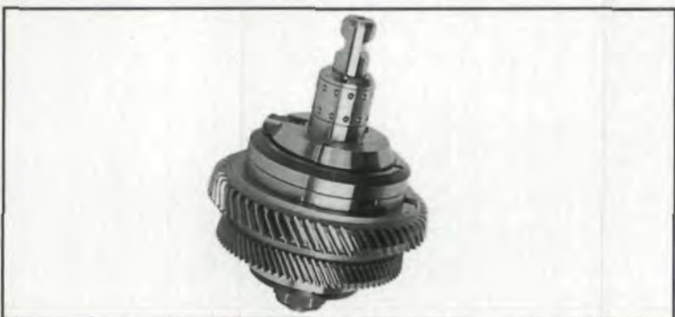
Fig. 23 — Cutter adapters are automatically clamped concentric to the cutter spindle to an accuracy of .0001-.0002". Two cutters are mounted for cluster gear cutting.
