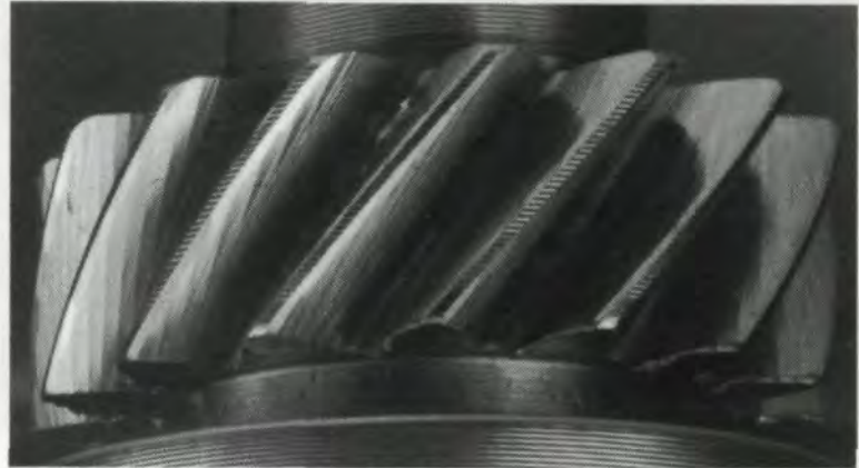
Fig. 19 — Feed marks and enveloping cut formation.
