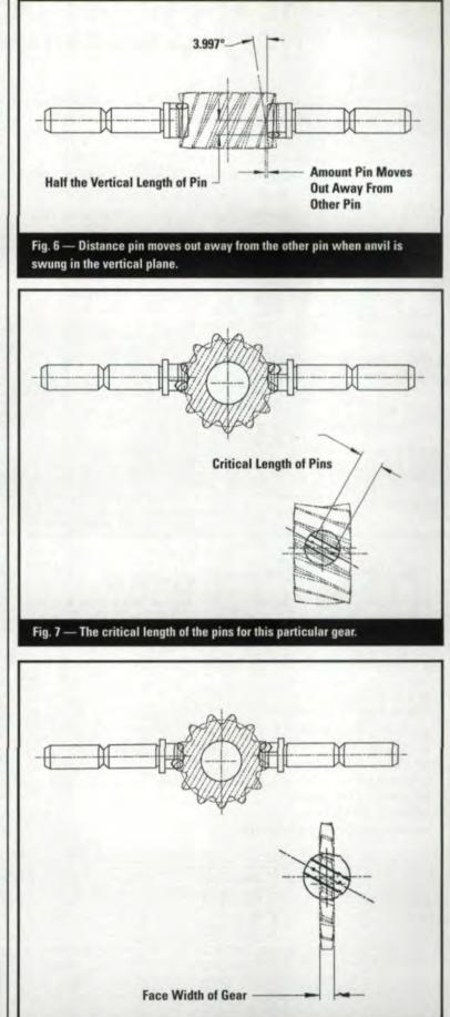
Fig. 8 — A gear where the limiting factor is the tooth length because it is less than the critical length of the pins.
