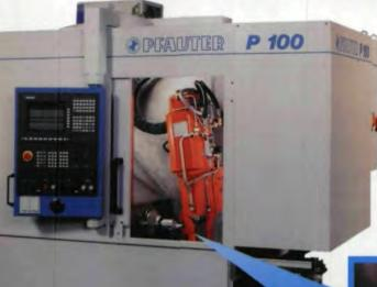
Introducing the revolutionary new P100 Horizontal Spindle, Direct Drive Hobbing Machine. Wet or dry, carbide or HSS... no matter how you cut it, automotive sun gears and pinions and high-production
