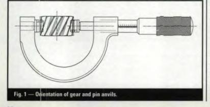
ally a "dimension over one ball" or a "dimension over one pin." To measure a gear over one ball or pin, an arbor is used to establish the center, which is the zero reference for the measurement. All external gears can be measured over one ball or over one pin.
