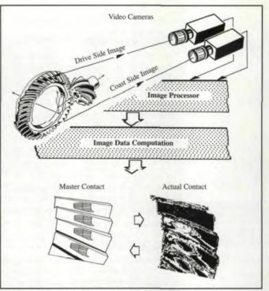
Fig. 4 — Contact recognition system by video image processing.
