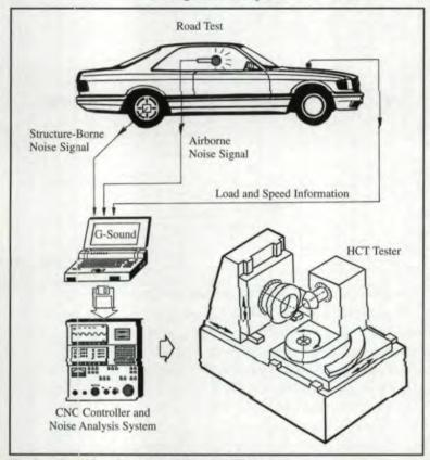
Fig. 6 — Closed loop between vehicle and HCT tester.
