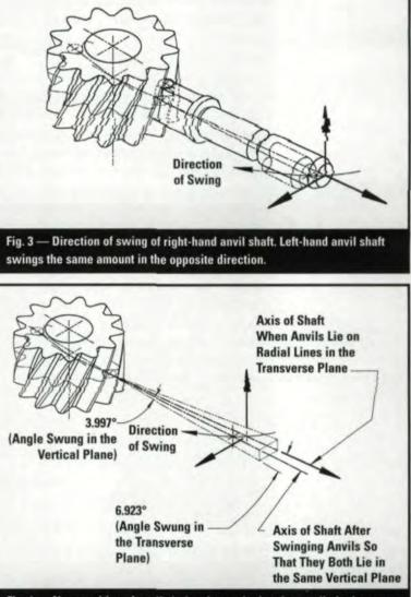
Fig. 4 — New position of anvil shafts after swinging them to lie in the same vertical plane.
