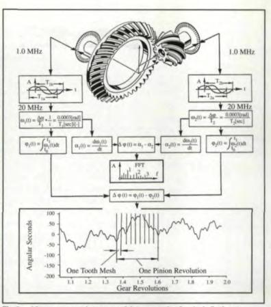
Fig. 2 — Measurement and structure of data processing for single flank tests. necessarily evident beforehand if criteria for all three test types can be established or if it is mandatory to do so.
