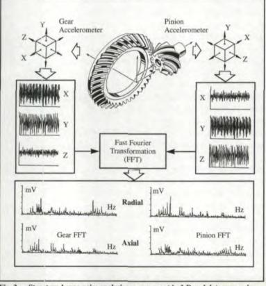
Fig. 3 — Structure-borne noise analysis measurement in 3-D and data processing.
