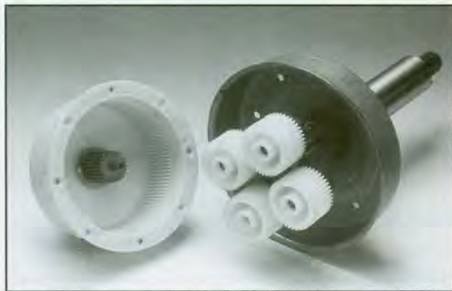
Fig. 2 — In the "World Washer," manufactured in several countries, Whirlpool Corporation introduced a splined clutch or "splutch," containing a spline and gears molded in acetal copolymer. The low-wear epicyclic gear assembly lasts four times normal washing machine life and reduces the number of moving parts by 20%.
