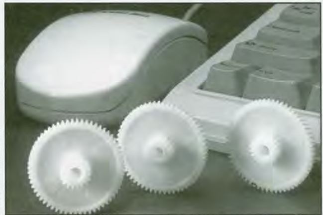
Fig. 1 — Hewlett-Packard took plastic gears to AGMA class Q9 to give its new color printer precise paper motion. For gears of this size, 1.25" in diameter and 48 pitch, the AGMA Class Q9 denotes gears with a Total Cumulative Error (TCE) of just 0.0015" and Tooth-To-Tooth (TTT) error of 0.00071".
