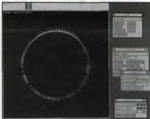
(Left) Fig. 3 — Looking down the long axis of the shaft, the data at the four levels is shown in one plane, and the deviations show that the shaft is tilted relative to its Z axis. Yellow whiskers turning to red (lower left) indicate that the shaft is larger than nominal on one side; on the opposite side of the shaft, (right in photo) blue whiskers indicate that the shaft is smaller than nominal at one depth, and yellow whiskers indicate that the shaft is larger than nominal at another height. This configuration is sometimes called the "banana" shape.
