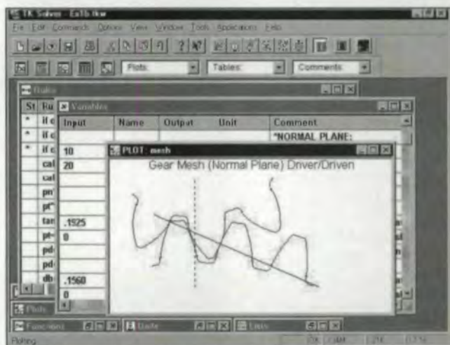
Universal Technical Systems now offers its programs for the Windows environment. Above: Program 60-411, Hob Cutting Pattern for External Involute Gear (top) and Program 60-400, External Gear Line of Action Tooth Plot (bottom).
