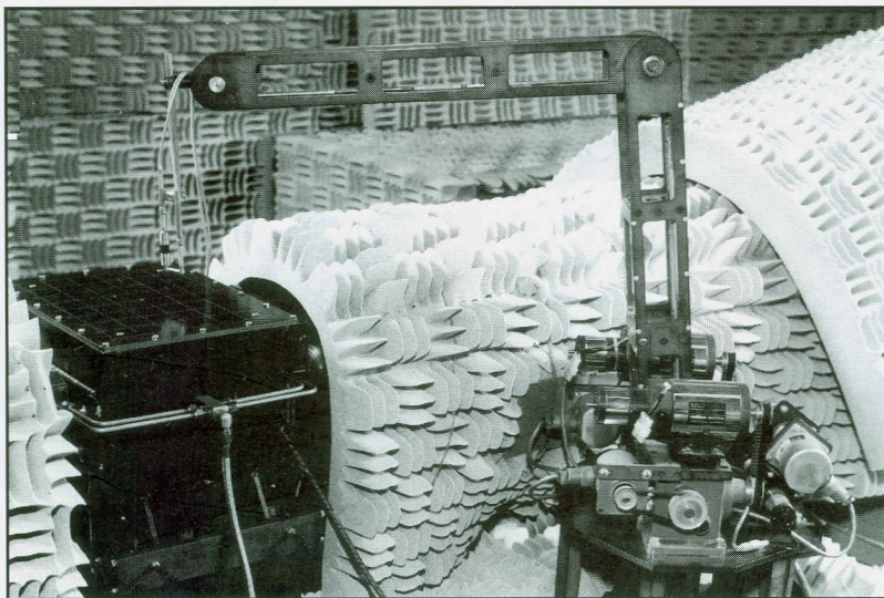
Fig. 3 — Test gearbox and RAIMS robot.
