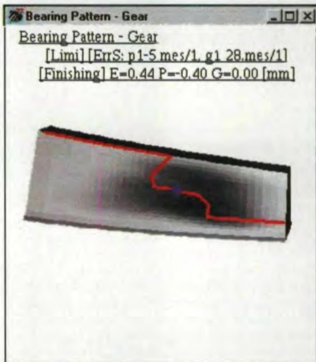
HyGEARS analyzes bearing pattern and tooth contact for spiral bevel and hypoid gear teeth.
