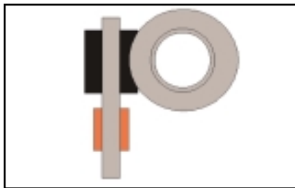
Figure 1—Teeth are hobbled into a gear in a normal cycle.
