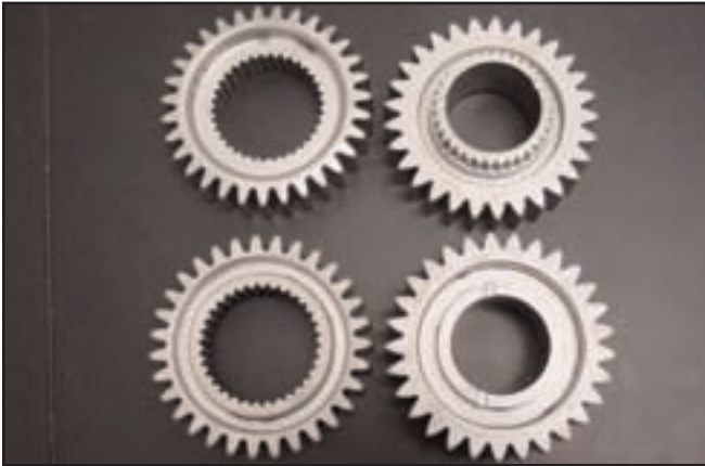
Figure 4—Racing transmission gear (AISI 9310).
