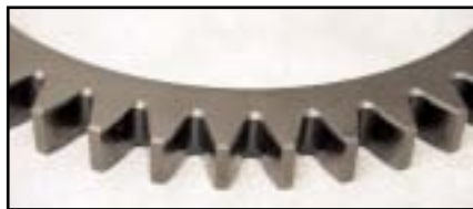
Figure 4—View of gear teeth with uniform chamfer as produced by chamfer hob.
