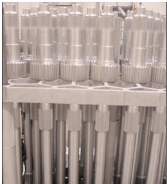
Figure 7—Racing transmission main shaft (AISI 4820).
