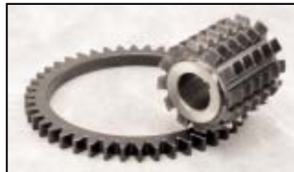
Figure 5—Chamfer hob shown with workpiece.
