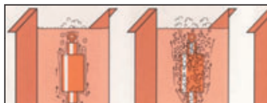
Figure 1—Schematic representation of the three stages of quenching for normal quench oil: 1) Left—vapor barrier formation; 2) Center—vapor barrier collapse and nucleate boiling; 3) Right—convection.
