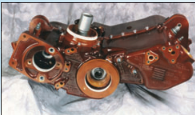
A gearbox from Arrow Gear Co. for the Joint Strike Fighter program.
