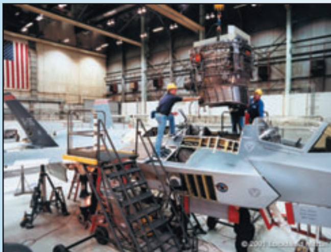
Installation of a Rolls-Royce Lift Fan System on a Joint Strike Fighter prototype. Courtesy of Rolls-Royce p/c.
