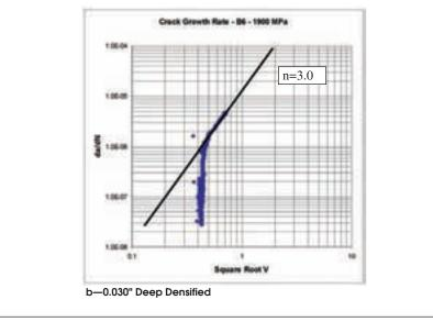
Figure 24—Crack propagation rate in FLN2-4405 surface-densified PM steel.
