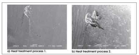
Figure 28—SEM of Ancorsteel 4300 after different carburizing processes.
