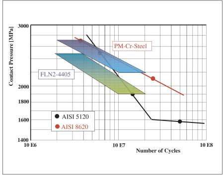
Figure 31—Comparison of surface-densified PM steels to wrought steels.
