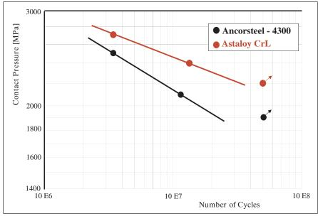
Figure 29—RCF strength of chromium-containing, surface-densified PM steels.
