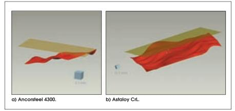
Figure 30-3-D CAD maps of first cracks in chromium-containing PM steels.
