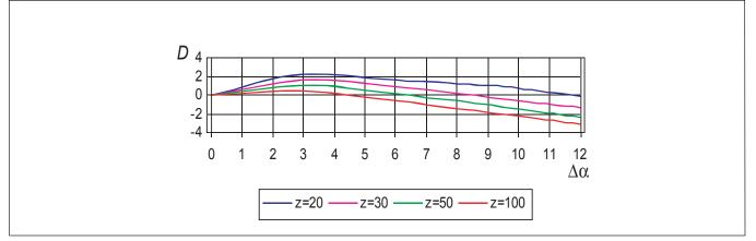
Figure 3—Difference D between the percentage stress reduction calculated using modified ISO C method and using FEM (x=0;  $\rho_{on}$ =0.25).
