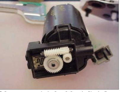
Plastic gears are now common in automotive applications such as this seat position sensor from ABA-PGT.
