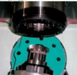
Kanzaki GSU180 internal gear shaving machine is a step forward in high precision gear finishing. You can now modify gear teeth profiles with high precision machining, helping reduce noise generated by automotive automatic transmission planetary gear systems.
