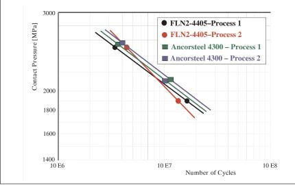
Figure 25—Effect of different carburizing cycles on RCF strength.FLN2-4405 and Ancorsteel 4300, both by Hoeganaes Corp. (Ref. 47).
