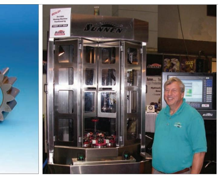
fully automated vertical machine—uses Sunnen's patented Krossgrinding® tools, which the manufacturer says are capable of controlling bore size down to 0.00005" and finish to 16 µin or better.
