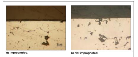
Figure 16—Failure mode in sinter-hardened PM Steel, density = 7.3 g/cm<sup>3</sup> (40).
