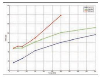
Figure 12—SPL versus speed and torque (second gear).
