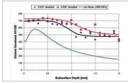
Figure 21—Microhardness and subsurface stress distribution.
