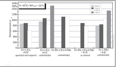
Figure 15-RCF strength of PM steels at different densities (Ref. 38).
