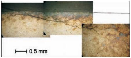
Figure 26-Crack path in Ancorsteel 4300.
