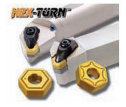
finish, even at high feed rates. The  $45^{\circ}$  lead angle allows high feed rates with low cutting forces. A  $120^{\circ}$  included angle provides a strong insert design and improved resistance against notching.
