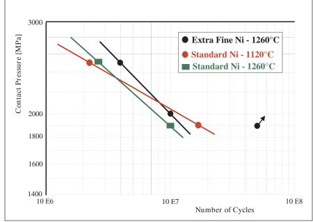
Figure 18—Effect of sinter temperature and nickel particle size on RCF of surface-densified PM steel FLN2-4405 (Ref. 43).
