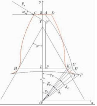
Figure 1—Comparison of symmetric (HCDKI) and asymmetric (HCAK'I') tooth forms.
