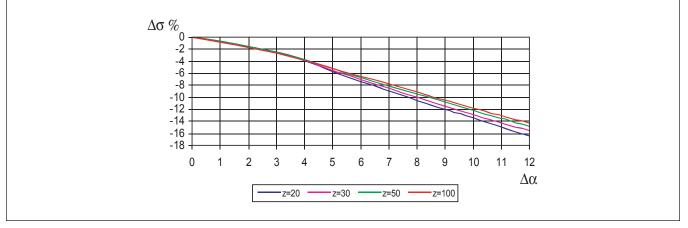
Figure 2—Percentage decrease of stress calculated using modified ISO C (x=0;  $\rho_{a0}$ =0.25).
