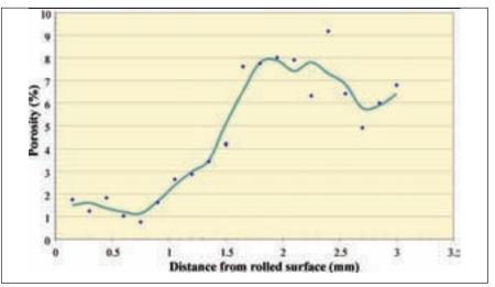
Figure 20—Porosity profile of surface-densified Ancorsteel 4300 (Ref. 47).
