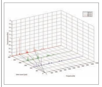
Figure 9—Sound pressure waterfall diagram (first gear).
