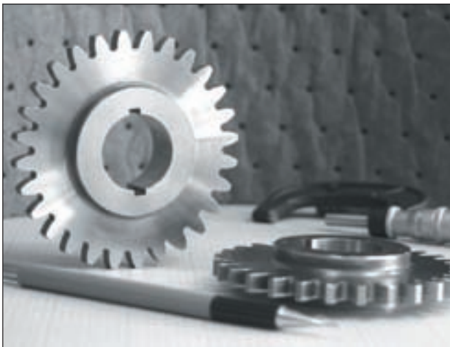
Figure 1—Gears for surface fatigue testing on the NASA Glenn Research Center gear fatigue test apparatus.
