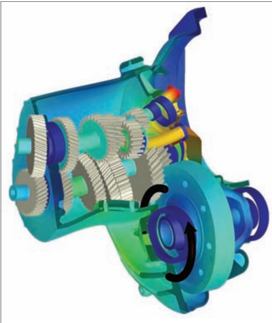
RomaxNVH: Exaggerated 3D view of a normal mode shape in a transaxle gearbox.
