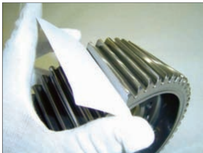
Figure 9—Close-up of a superfinished gear.
