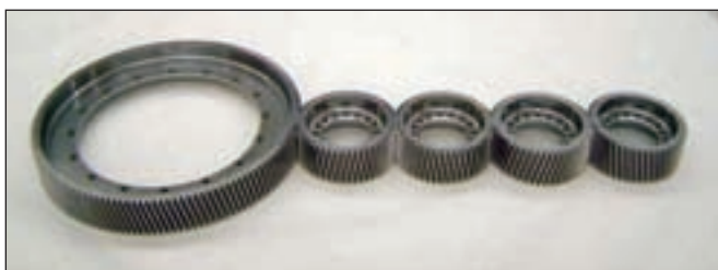
Figure 8—Entire gear train after superfinishing.
