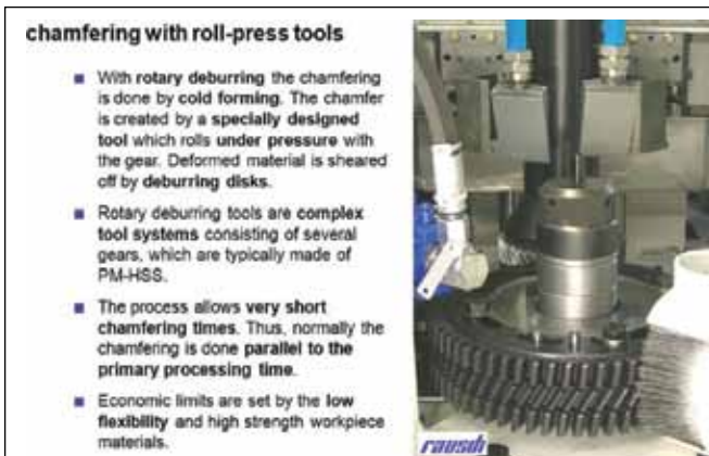
Figure 10—Rotary deburring.
