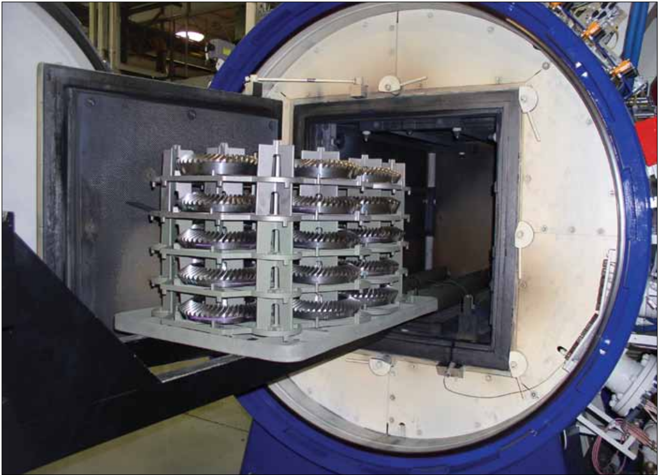
Vacuum carburizing offers shorter cycle times and better quality control compared to traditional heat treat methods (courtesy of Ipsen).
