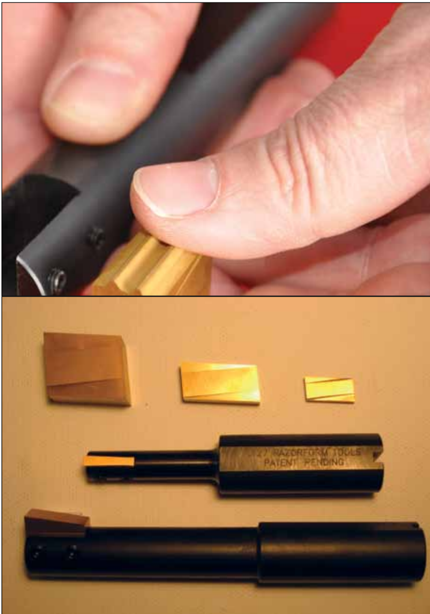
Razorform Tools carbide inserts remain in the machine turret during indexing, resulting in longer tool life while reducing downtime.
