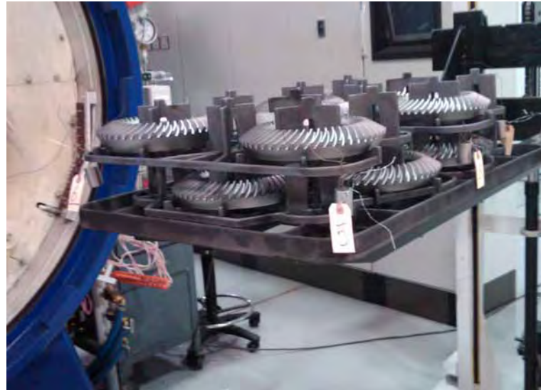
Test load of ring gears for a customer order (courtesy of Ipsen).
