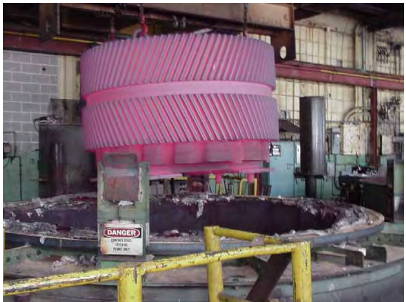
A 39,000 pound gear is lifted out of the carburizing furnace (courtesy of Metlab).
