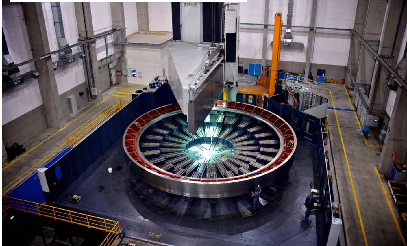
Ferry Capitain's recently commissioned VBCM16 is capable of turning and cutting gears up to 16 meters in diameter with 1,200 mm face width and 350 tons on the table.
