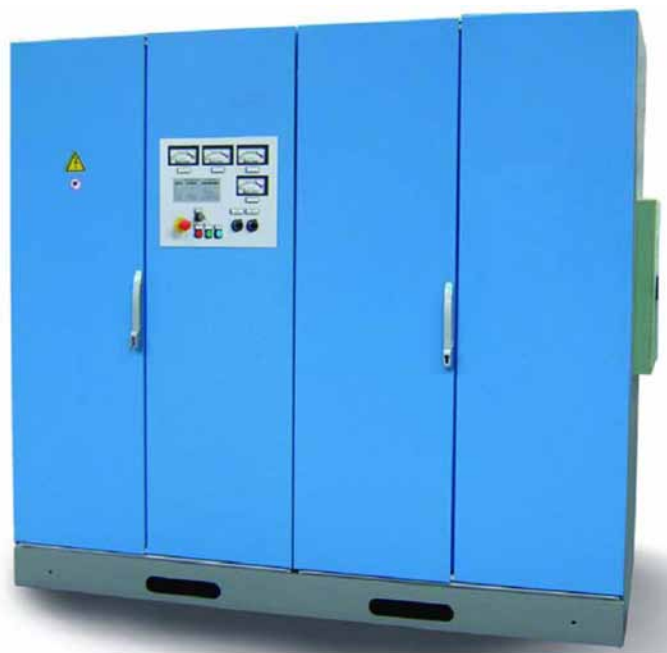
Figure 3 Inductoheat's Statipower IFP is an IGBT-type power supply specifically designed for induction hardening and tempering applications; it provides independently adjustable frequency via CNC programming in a 5–40 kHz frequency range and power in the range of 10–360 kW.
