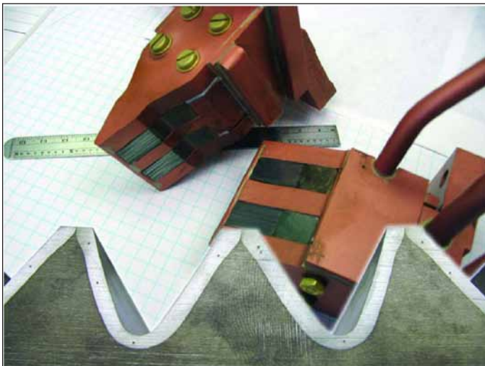
Figure 1 For tooth-by-tooth hardening, inductors can be designed to selectively harden specific areas of gear teeth where metallurgical changes are required (Ref. 2).
