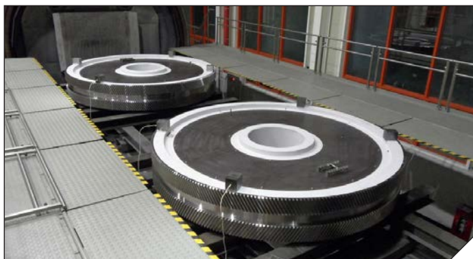
Figure 1 Large steel gears for the shipping industry weighing multiple tons and 8.8 feet (3 meters) in diameter have been wear-protected with the PPD solution (all photos courtesy Oerlikon Balzers).
