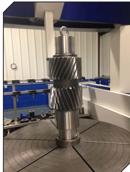
Brad Foote converted its processes for the pinion and bull gear to utilize the Cubitron II wheel. The company has also begun implementation of the wheels for additional grinding applications in the mining industry.
