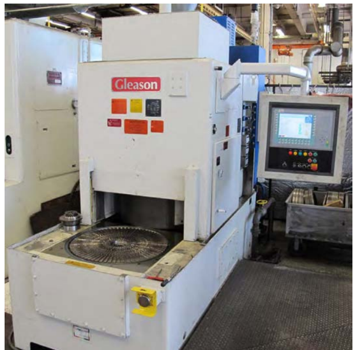
Figure 1 A modern quenching machine (All images courtesy The Gleason Works).
