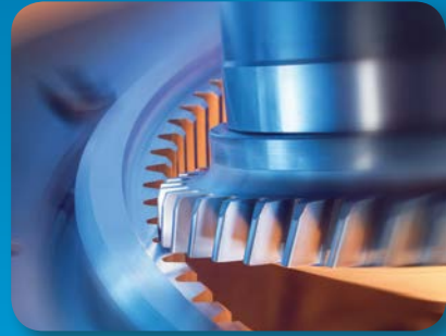
Production of cylindrical gears up to 600 mm in diameter, swing diameters to 750 mm and modules up to 6 mm.
