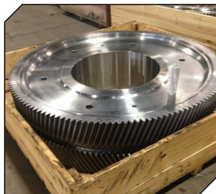
The photo shown here is not the bull gear being discussed, but is included as an example of what happens to this type of material with the incorrect tooling or grinding strategy (all photos courtesy of Brad Foote).
