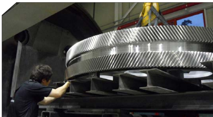
Figure 1 Large steel gears for the shipping industry weighing multiple tons and 8.8 feet (3 meters) in diameter have been wear-protected with the PPD solution (all photos courtesy Oerlikon Balzers).
