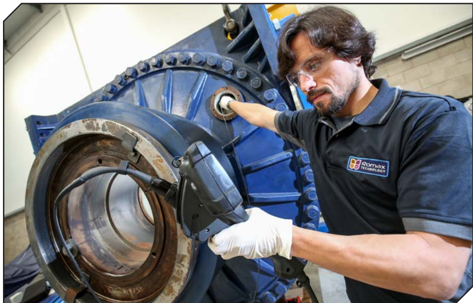
Determining root failure cause: Endoscope inspection of a wind turbine gearbox.
