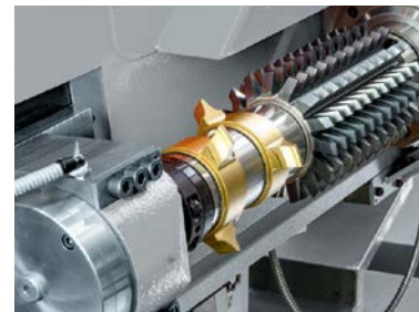
Chamfering in the work area
