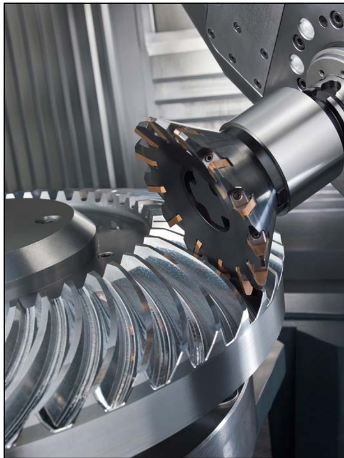
Figure 1 New technologies have converged to finally make it practical to apply 5-axis machining for production of many different gear types, all with high quality.
