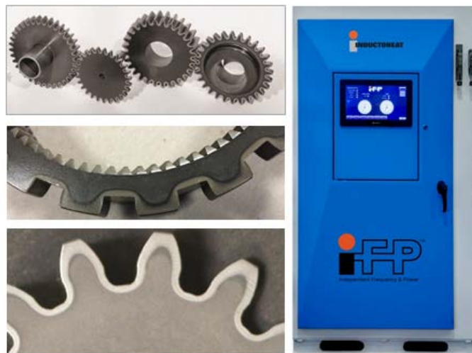
Figure 2 Statipower IFP Technology enables instant and independent adjustment of frequency within 5 to 60 kilohertz range in a preprogrammed manner during the heating cycle. (Photo courtesy of Inductoheat Inc.)
