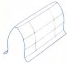
4 combination of (2) longitudinal correction and (3) uniform modified profile
