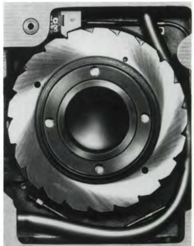
Fig. 11—Mechanical indexing head (CNC indexing is also used).
