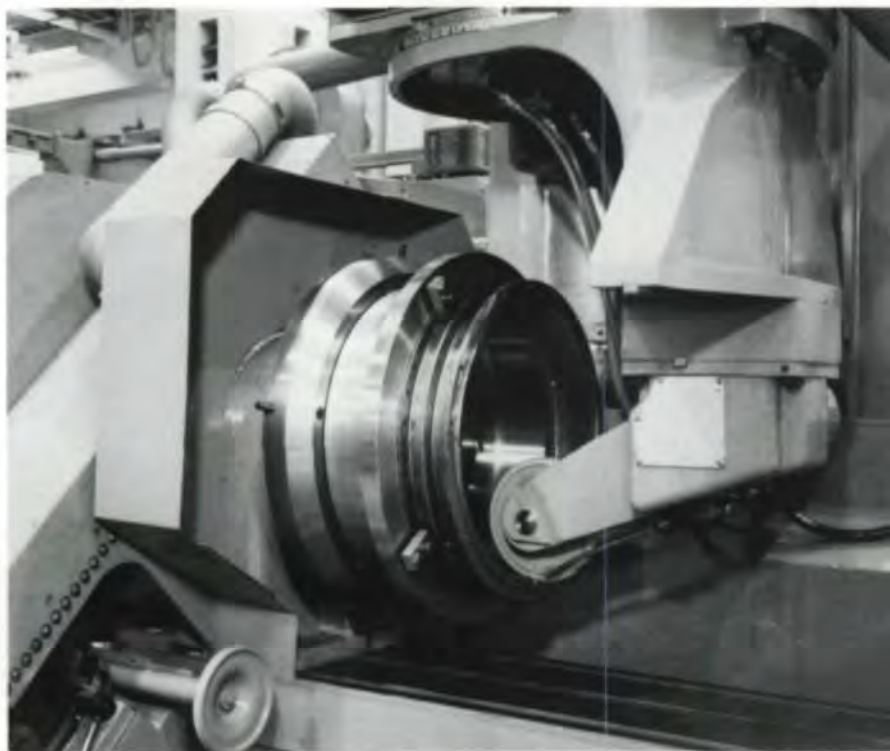
Fig. 9B - Form grinding on internal ring gear.
