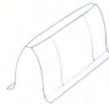
2 crowning (longitudinal corrections) with plain involute tooth profile
