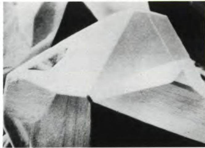
Fig. 21—Cubic boron nitride grain.
