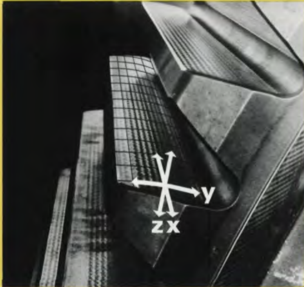
Fig. 25—NEW: Topological Modification variable modification "Z" of tooth profile across facewidth "X" as well as along profile "Y".
