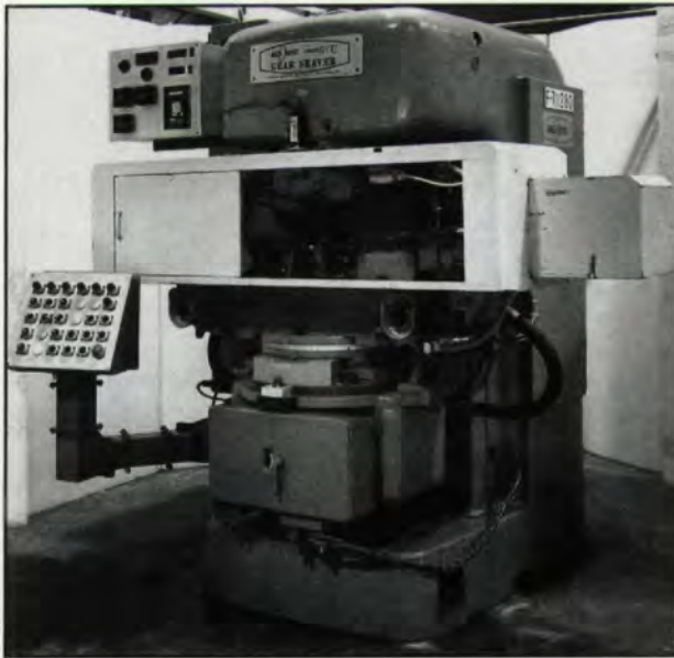
Fig. 4 - 12" Rotary gear shaving machine.
