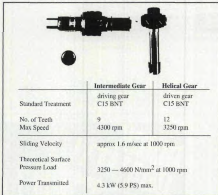
Fig. 1 — Investigated pair of gears.
