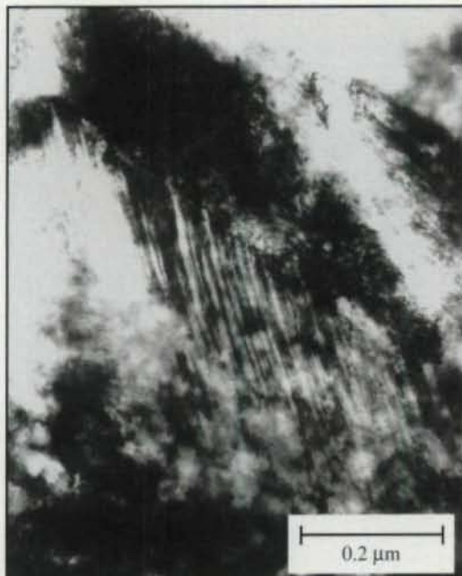
Fig. 4a — Ausrolled microtwins.
