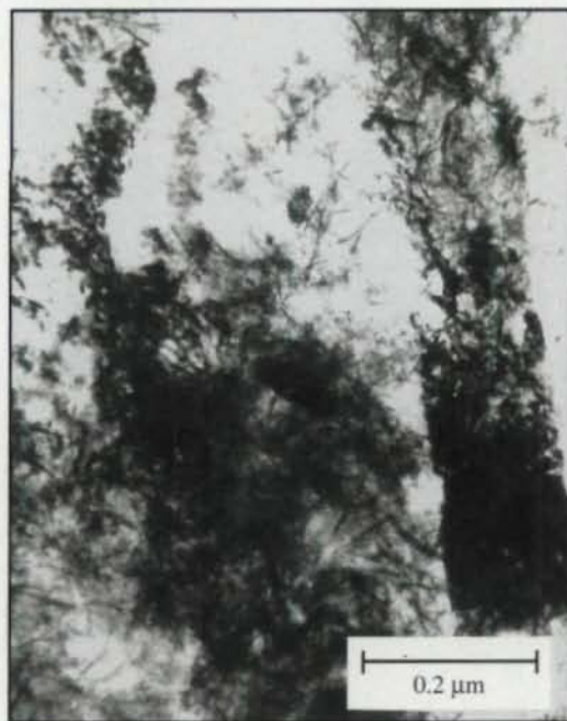
Fig. 4b — Ausrolled dislocations inherited by martensite.
