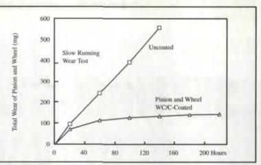
Fig. 5 — Wear test for a slow running gear for a concrete mixer. Stress: 2180 MPa. Sliding velocity: 0.04 m/s.
