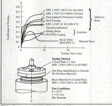
Fig. 3 - Dry running properties of friction materials.
