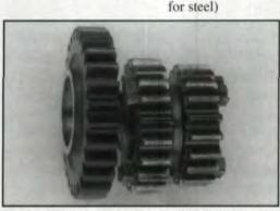
Fig. 4 - Wear of motorcycle gear after oil leakage during a race. Right: uncoated. Left: WC/C-coated.
