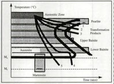
Fig. 4 — Lengthening the holding time.
