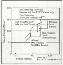
Fig. 6 - Surface fatigue strength of materials for gears.
