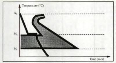
Fig. 3 - Cooling curve using graded hardening.
