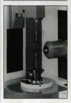
CNC Gear Measuring Centers Klingelnberg introduces its new PNC 33 Gear Measuring Center. The smallfootprint, 13" capacity, 4-axis machine
