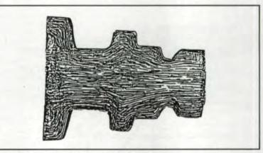
Fig. 1 — The correct distribution of fibers in a gear.
