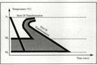
Fig. 2 - Cooling curve.
