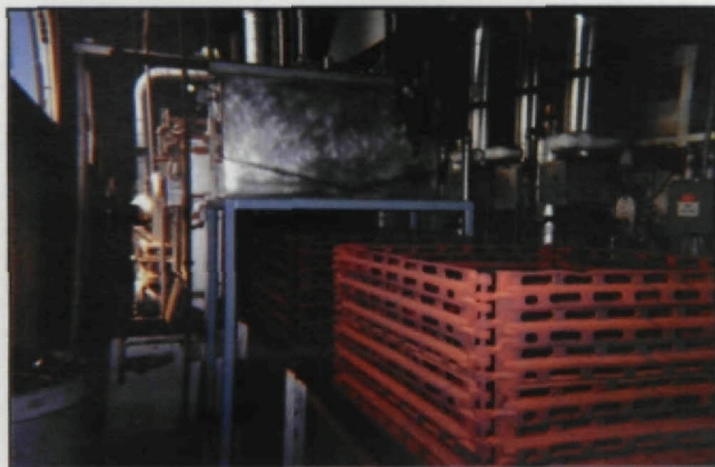
Fig. 1 — Treat-All Metals deployed a gravity separator above the parts washer conveyor line. Oily surface solution is pumped up from the wash tank by direct suction skimming. Oil and grit are removed in the separator (center, top). Clean, oil-free wash solution is continuously recycled back to the wash tank.
