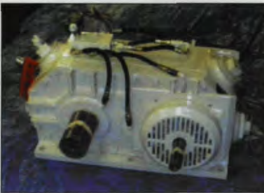
Figure 5—External lubrication system with hydraulic hose.
