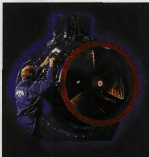
An employee of ATA Gears Ltd. works on one of the company's water turbines. The turbines are usually used by energy-producing companies and private companies that own river rapids.
