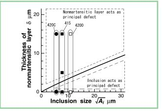
Figure 10—Comparison of the influence of the inclusion size and the thickness of nonmartensitic layer.
