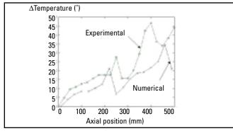
Figure 6—Temperature variations versus axial position—Case 2. with r = R/M as fluid constant, R as molar constant (8.3144 J.mole<sup>-1</sup> K<sup>-1</sup>) and M as molar mass.
