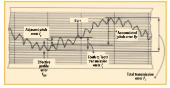
Figure 4—Individual errors revealed by single-flank testing.
