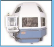
other ground parts. The machine's concept is to produce a complete workpiece by spreading the grinding operations over up to five different grinding stations on the same machine. The cycle time to produce a ground part is equal to the longest single operation plus transfer time.
