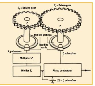
Figure 3—The principle of a single-flank measuring machine.
