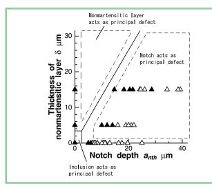
Figure 14—Comparison of the influence of the notch depth and the thickness of the nonmartensitic layer when the inclusion exists.
