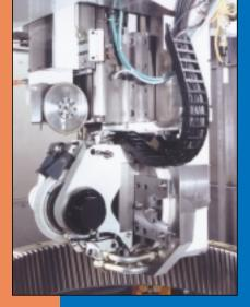
Setup measured in minutes vs. hours is Gleason's new patent-pending software, which automatically compensates for clamping misalignments and eliminates the possibility of both radial eccentricity and axial runout after the setup.
