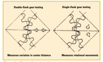
Figure 1—Composite gear testing.
