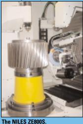
Overton Gear specializes in short runs and quick delivery of high-quality cut and ground gears for locomotives, off-highway vehicles, wind power turbines, industrial extruders and other heavy machinery. The company can cut either internal or external spur or helical gears from 12 mm (1/2") up to 2 m (80") in diameter, and it can grind internal gears up to 1.2 m (47") and external gears up to 1.5 m (60"). Overton Gear also has its own in-house heat treating facility.
