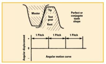
Figure 5a—A perfect involute tooth showing zero angular displacement error.
