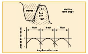
Figure 5b—An involute tooth with tip and root relief that result in parabola-like motion curves.
