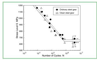
Figure 8—S-N curves in 4200 gears and 420C gears.
