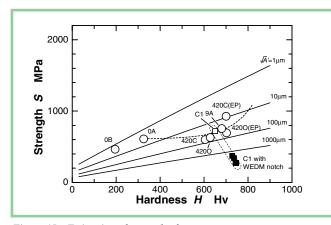
obtained by the microscopic observation is, however, scattered in a rather wide range as illustrated in the figure. So, the actual size of the inclusion which caused the tooth breakage is not clarified, and this may be the above mentioned result. This figure quantitatively shows the effectiveness of tooth surface finishing in enhancing the strength.
