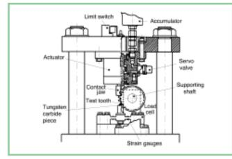
Figure 7—Pulsating fatigue test rig.
