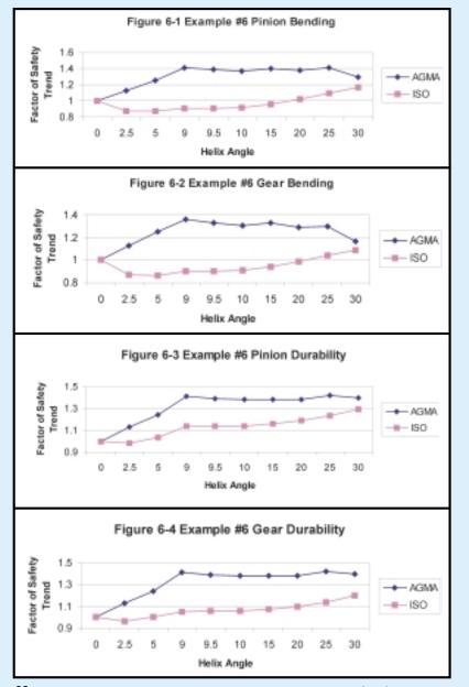
helix angle increases, the rating differences are influenced by both the helix angle changes and the increases in sizes for the gearing. For this reason, a new example was developed where the center distance was held constant when the helix angle was changed. This required that the transverse pitch/module be kept constant. This requires that the normal pitch/module be changed when the pressure angle changes.
