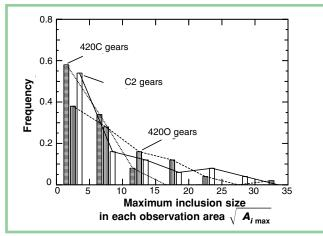
Figure 5—Distribution of the maximum inclusion size in each observed area.
