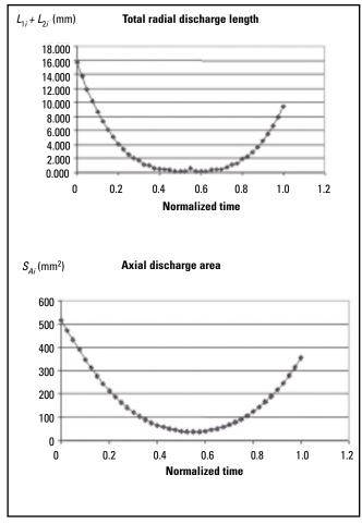
Figure 3—Evolution of radial clearances and axial exit area.
