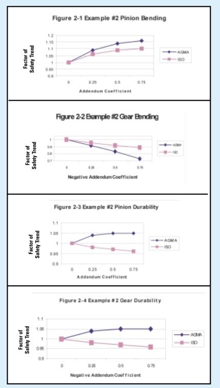
21 teeth on the pinion 84 teeth on the gear 5 module (5.08 normal diametral pitch) 20° pressure angle 100 mm (3.939") face width Standard hob proportions are being used Center Distance = 262.5 mm (10.3346")
