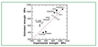
Figure 11—Estimation of strength of gears based on the defect size.
