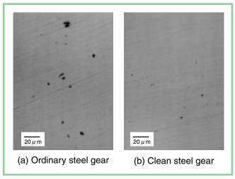
Figure 3—Microstructure of the ordinary steel and clean steel by optical microscope.
