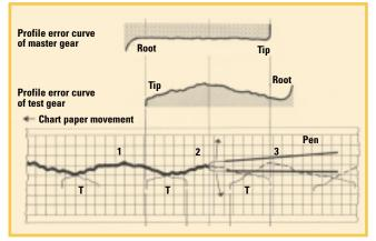
Figure 6—Direct relationship between an involute tooth and a single-flank graph.
