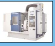
(1.97"), and module range of 0.5 to 4.5. The ZH 200 can combine its high cutting speeds with an optional, fast, fully integrated gantry loader system, thus offering the potential for significant improvements in overall cycle times.
