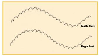
showing zero angular displacement error. Figure 5b shows gradual tip and root relief, typical of shaving operations, that result in the parabola-like motion curve. Figure 5c shows a tooth with pressure angle error and the resulting saw tooth motion curve.
