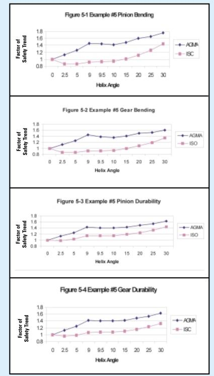
safety for both the pinion and the gear are lower for a helical gear than for a spur gear until the helix angle reaches  $15^{\circ}$  on this sample gear set. In AGMA, the factors of safety for bending on both the pinion and the gear in this gear set are lower between the value for the helix angle that has a helical overlap greater than 1.0 and a helix angle of  $15^{\circ}$ .
