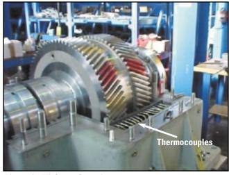
Figure 4—High speed test rig.
