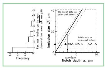
Figure 12—Comparison of the influence of the notch depth and the inclusion size.
