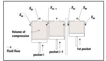
Figure 2—Discrete hydrodynamic model for helical gears.
