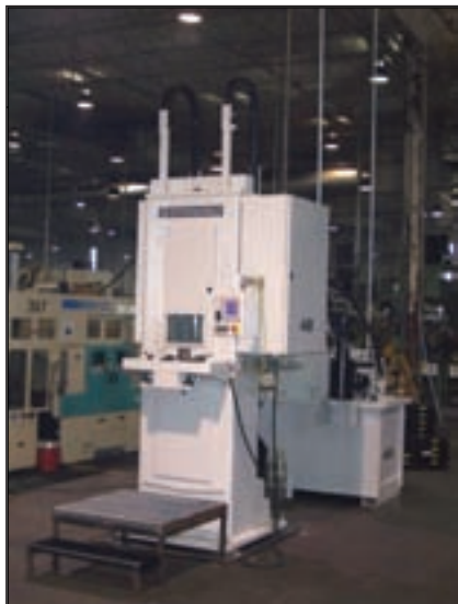
MVS Metform in Savanna, IL, recently installed a new Stenhøj broaching machine.
