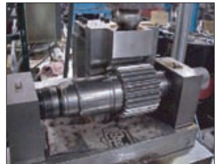
Figure 4—Single-tooth fatigue fixture.
