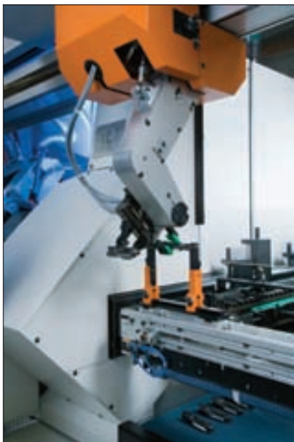
The integral gantry loader with rotating twin-gripper allows for shortest loading and unloading times.
