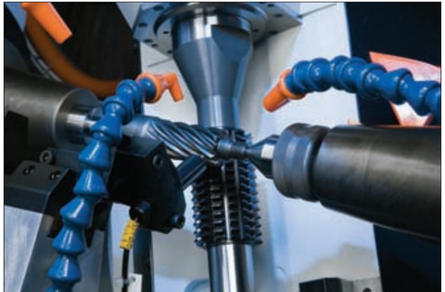
The Koepfer 160 gear hobbing machine is well-suited to manufacture steering pinions with an eight-axis control system and high speeds on both the work and cutter spindles.
