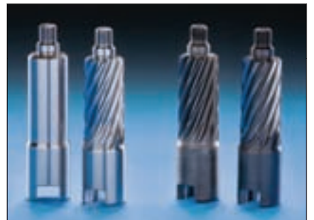
The K160 manufactures steering pinions by soft pre-hobbing and hard finish-hobbing (skiving) of the gearing.
