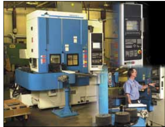
Eurotech-Famar CNC Pronto 5 Turning Cells features Siemens controls, drive and spindle package.
