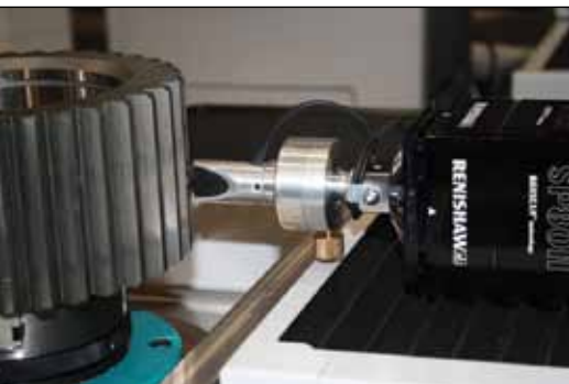
The Wenzel WGT 500 gear measuring machine is equipped with Stresstech Rollscan R500 Barkhausen noise analyzer System integrated with a horizontally-mounted Renishaw SP80 probe.
