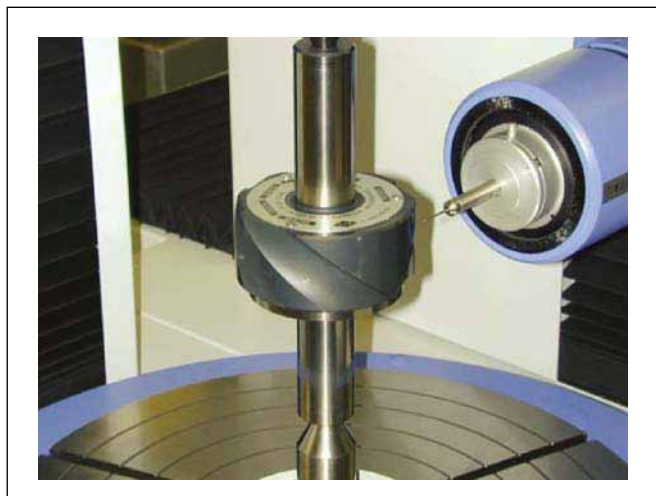
Figure 6—Traditional Fellows-type helix (lead) artifact.
