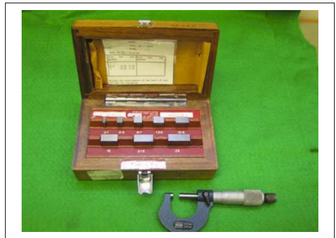
Figure 3—Micrometer and M8-gauge block set used for functional micrometer calibration.
