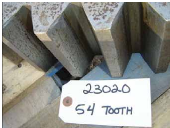
Figure 3—Used 54-tooth, 1.5-pitch gear rejected for further service, yet also having been pulled in this condition from a working jacking system (courtesy ESI, Inc.).
