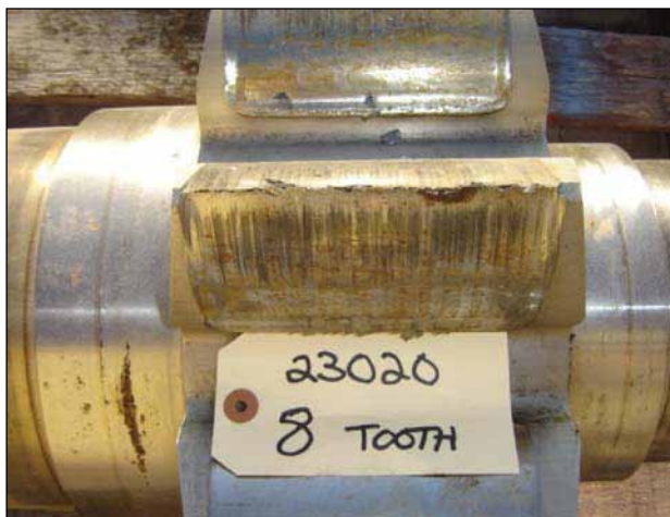
Figure 1—Used 8-tooth, 2/3-pitch pinion, rejected for further service, yet having been pulled in this condition from a working jacking system (courtesy ESI, Inc.).
