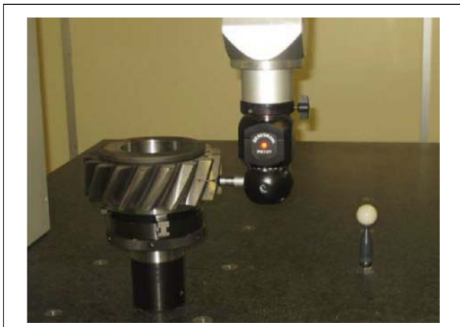
Figure 1—CMM used for gear measurement.
