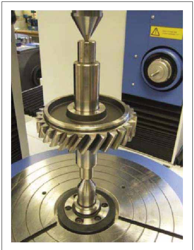
Figure 12—M5 master trial gear.
