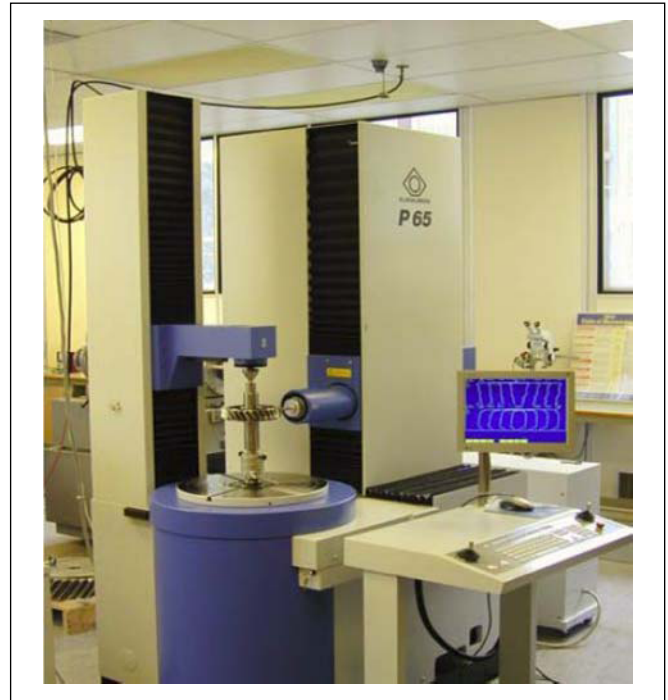
Figure 2—Example GMM: the U.K. primary gear measuring machine.
