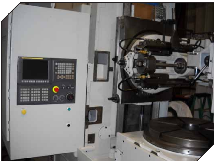
A mechanical (change gear-driven) Modul ZFWZ800 gear hobbing machine that was fully rebuilt and re-controlled to have four axes and one spindle under CNC control. The CNC was Fanuc model Oi-MD (Courtesy MTB).
