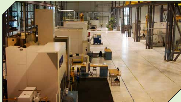
A partial view of the 105,000 square foot Brevini Wind manufacturing facility. The company broke ground on the facility in 2009 and began installing equipment by late 2010/early 2011. The facility also houses a 6.4 MW capacity back-to-back test bench for full load testing of large planetary gearboxes.
