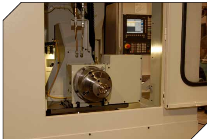
A fully re-built Lorenz LS-180 gear shaping machine that had a custom tailstock/face gear table assembly added to it during the re-build. This machine has five axes of CNC control and one spindle — all controlled by a Siemens 840D CNC (Courtesy MTB).
