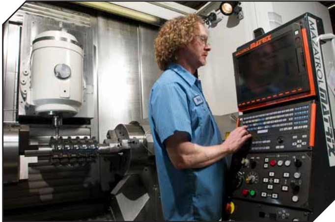
Gleason's coarse pitch hob cell machines tools complete from barstock, even on hobs as large as 450 mm diameter, 530 mm in length and up to 40 module, to achieve 6-week deliveries.
