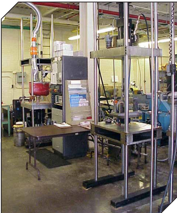
Single-tooth fixture equipment used for bending fatigue testing
