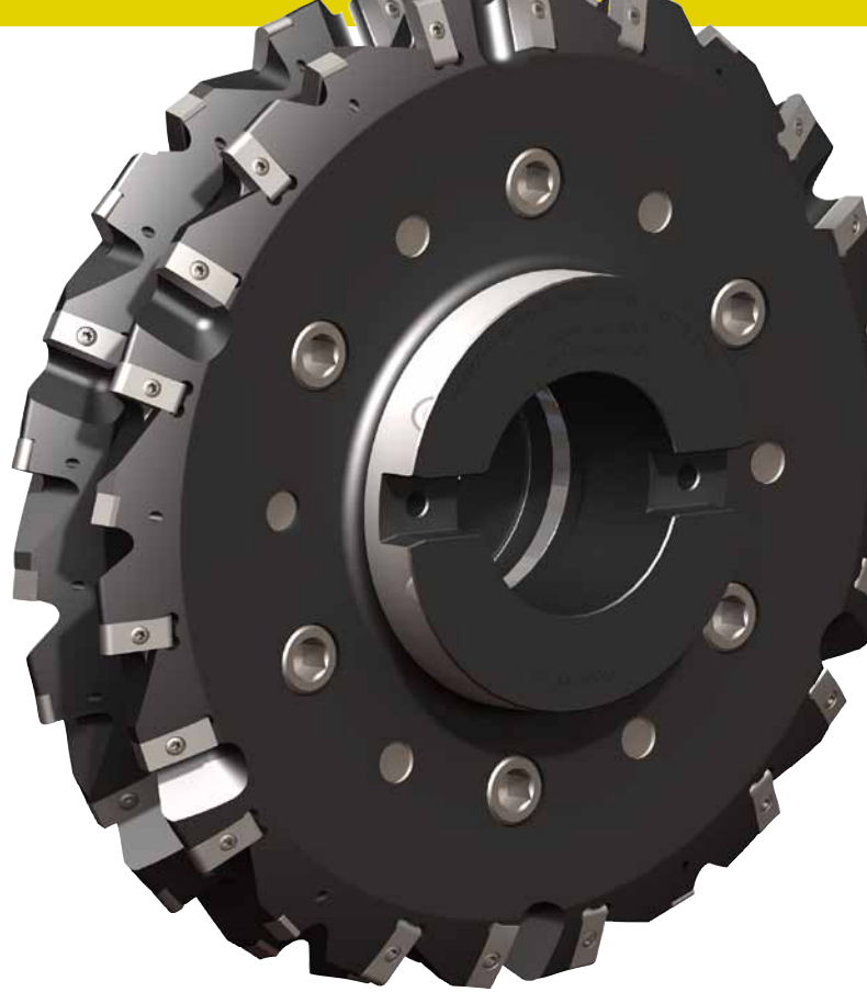
A rendering of the duplex profile milling cutter used to generate the semi-finished gear geometry of the 12-module gear. Profile milling using the duplex cutter resulted in a total cutting time of under 55 minutes for the 76-tooth, 282mm face width gear. (image courtesy of Banyan Global Technologies)
