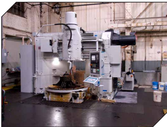
A mechanical shaper that was fully re-built, modified and converted to CNC control. It has five axes under CNC control, using a Siemens 840D CNC. It was modified to use a 2000 Nm water-cooled torque motor to generate the up/down stroking motions. The upgrade also provided CNC-controlled elevation adjustment and high-speed return of the cutter, helping to reduce cycle time from seven to two hours on most parts (Courtesy MTB).
