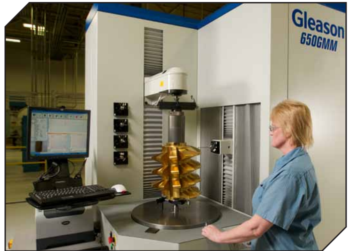
Every operation is totally integrated, even the final step: complete inspection of all critical features on a Gleason GMM analytical gear inspection system.
