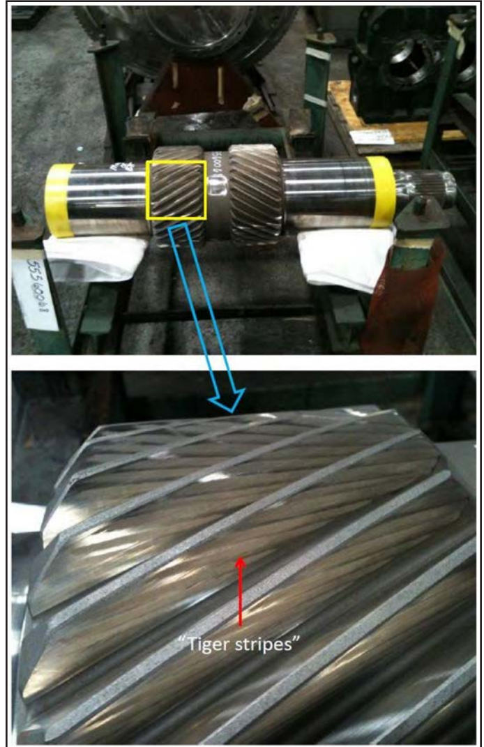
Figure 1 Tiger stripes on the pinion.
