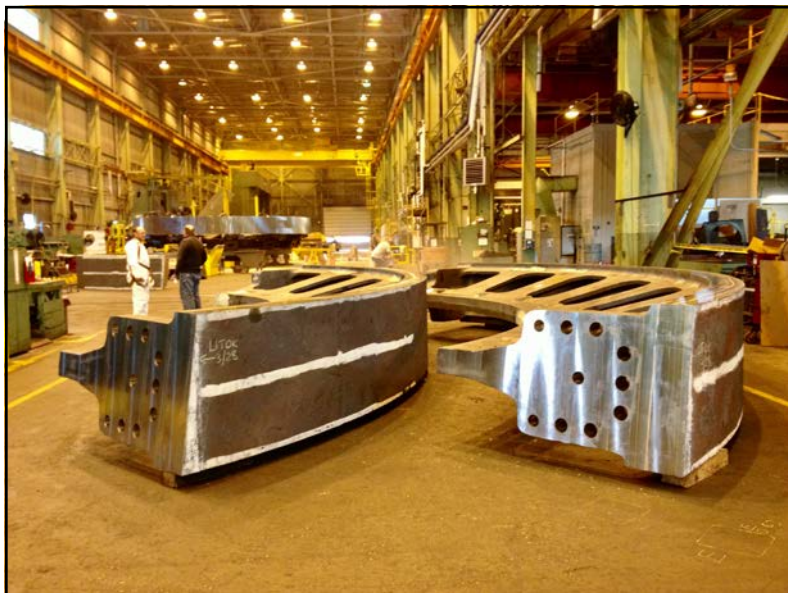
Figure 5 Unassembled segments for 34' (10.5 meters) 4-piece girth gear.
