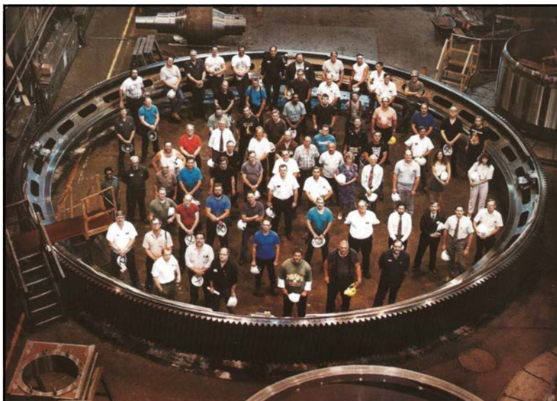
Figure 6 Finished 40' (12 meter) 4-piece girth gear.
