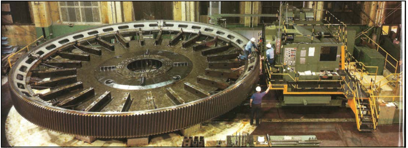
Figure 2 Girth gears exceeding 24 feet typically require up to six segments.
