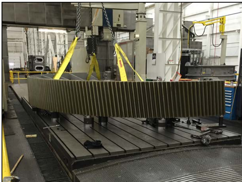
Figure 4 Prepping girth gear segment for reworking.
