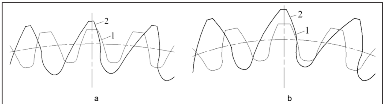
Figure 10 Metal (1) and asymmetric plastic (2) gear tooth profile comparison; a – pinion teeth, b – gear teeth.
