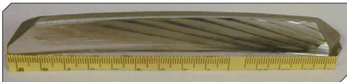
Figure 1 An example of tiger stripes failure (this image appeared as Fig. 2a in Ref. 1).
