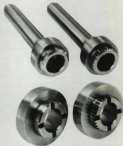
Typical parts before and after splines are broached. Splines can be external, internal, or both.
