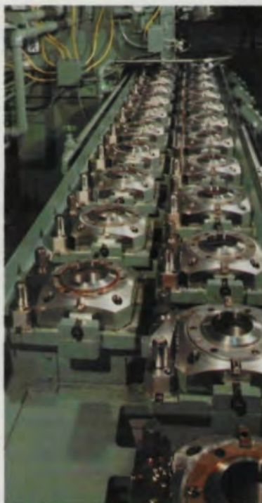
Progressive tooling for two different parts. Spline surfaces are broached within 0.001-in. TIR from locating surfaces.
