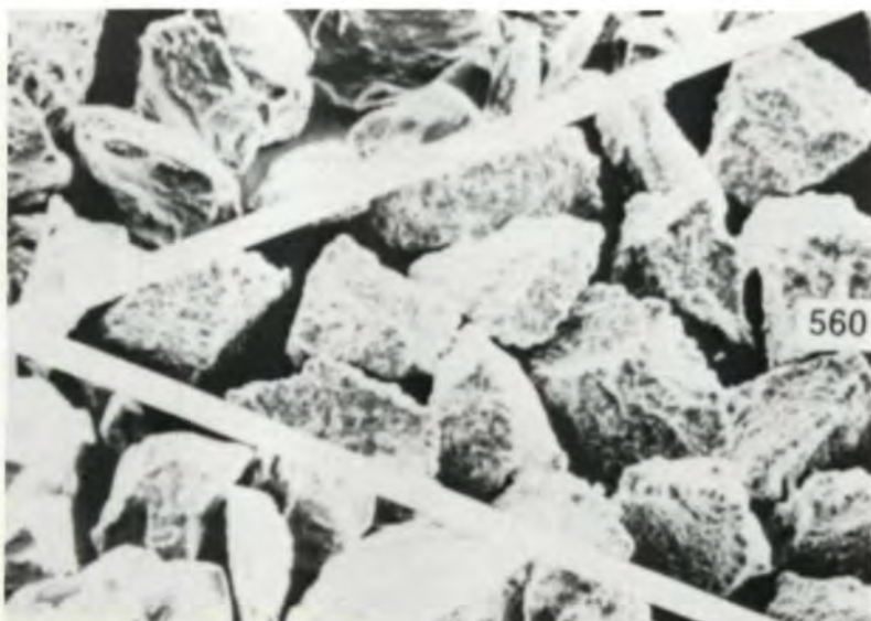
Fig. 2—Typical crystals of cubic boron nitride.
