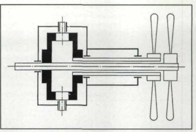
Fig. 9 - Coaxial counter-rotating propellers.
