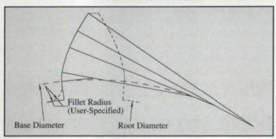
Fig. 2 - Typical EDM gear involute.
