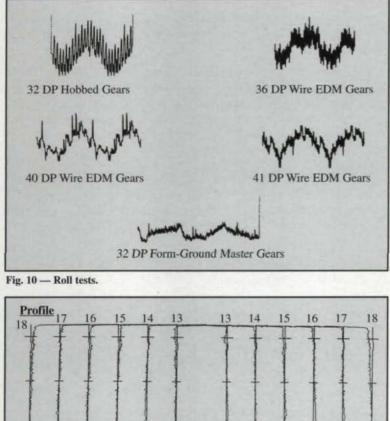
7 QCL12 2 Ff 2 2 2 2 3 2 -2 fHA 1 2 2 ff Runout fr fr = 2Spacing fp1 fp = 1fp2 =fp = 1**Gear Data** N = 19TTp = .34414Ff = Transverse Profile Total Deviation DP = 5OD = 4.3732fHA = Transverse Profile Angle Deviation  $\Phi = 20^{\circ}$ FD = 3.58279 ff = Profile Form Deviation Fr = Total Runout Deviation fp = Adjacent Pitch Deviation
