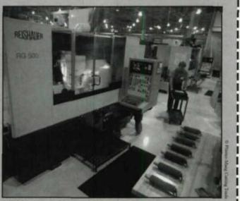
A finish grinder in Plauter-Maag's carbide cell.
