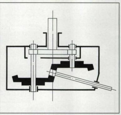
Fig. 14 - Helicopter gear assemblies. (Patented by Lucas Western, Inc.)
