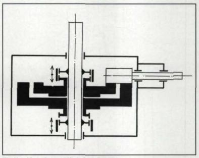
Fig. 10 - Ninety degrees (90°) dual-speed gearbox.
