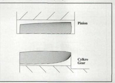
Fig. 3 - Lines of contact at the pinion and the Cylkro gear flank.
