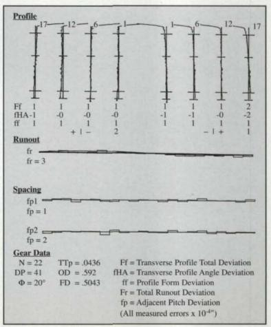
This 5 DP gear satisfies the criteria for a Class 2 master gear, with similar cost and production advantages over form-ground gears.
