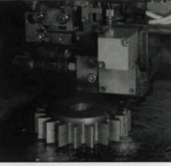
Fig. 1 — Wire EDM gear cutting setup.
