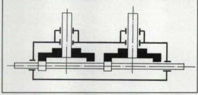
Fig. 7 - Centrally driven shaft with several distribution points.
